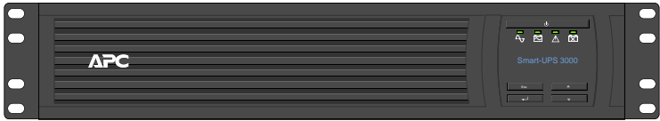
RACK MOUNT UPS. L5-30 INPUT. L5-30 OUTPUT. CAPACITY NTE 2880 VA. 2 RU. METERED (APC SMX3000ORMLV2U OR EQUIVALENT)
