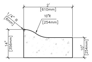
NOTE: CROSS SLOPE OF GUTTER SAME AS PAVEMENT.
