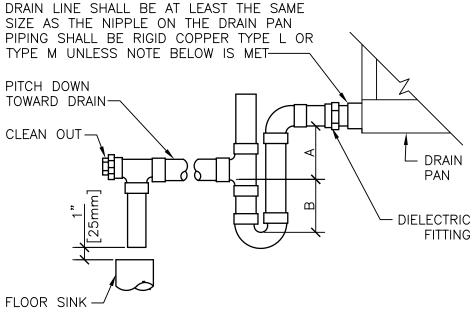
1. CPVC PIPE MAY BE USED ONLY IF APPROVED BY LOCAL VA AND IS INDOORS AND DOES NOT PASS THROUGH RATED BARRIERS.
