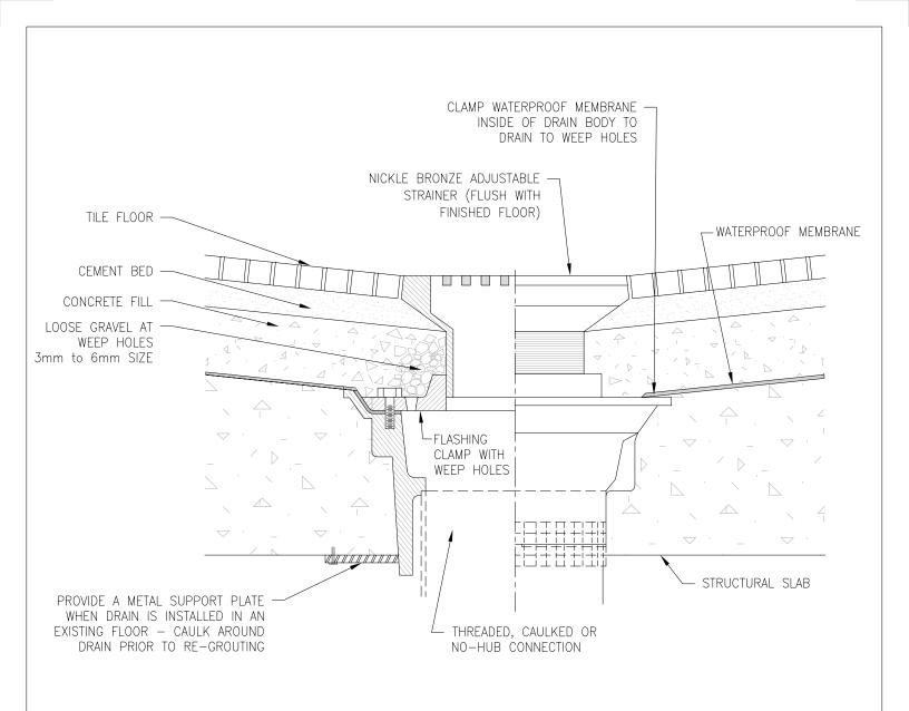
NOTE: SLOPE MEMBRANE LINER 2% TO DRAIN.
