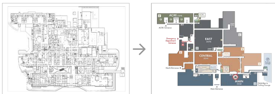
Figure 1-18 A wayfinding master plan reduces the complexity of information and simplifies the wayfinding experience by creating a logical structure of the space.
