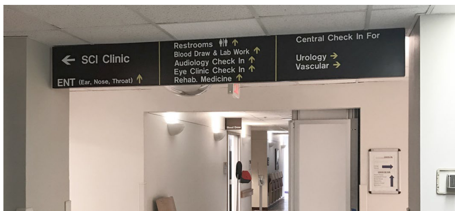
Figure 1-7 (Right) The overhead sign is confusing because it lists too many destinations and the directional arrows are used incorrectly. To minimize confusion, overhead signs should only include a limited number of major destinations. Additionally, a single directional arrow pointing in the direction of travel should be used in combination with wall-mounted signs that provide more detailed information.
