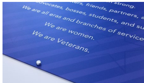
Figure 1-34 Wide-format digital printers allow for greater flexibility in design and low VOCs in comparison to silk-screening or painting. They also allow for surface or subsurface printing directly to the substrate
