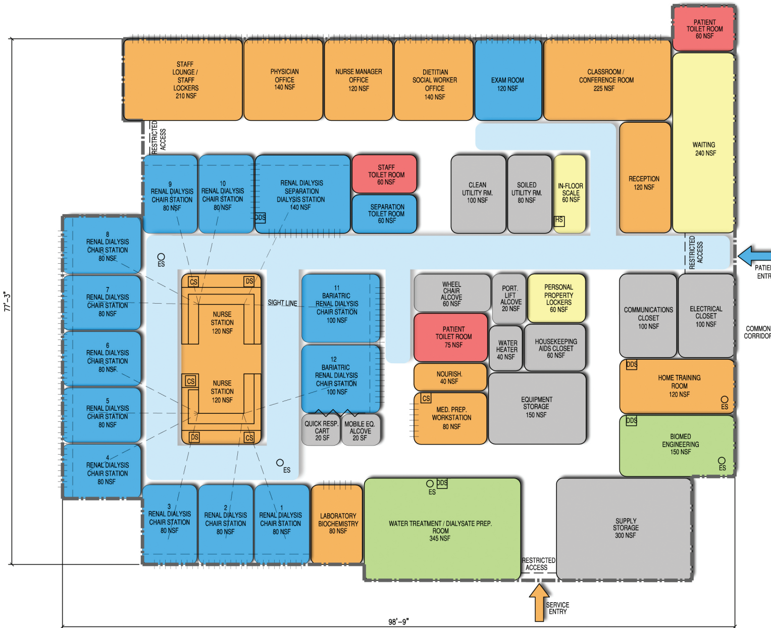
12 - STATION DIALYSIS CENTER BUBBLE DIAGRAM
