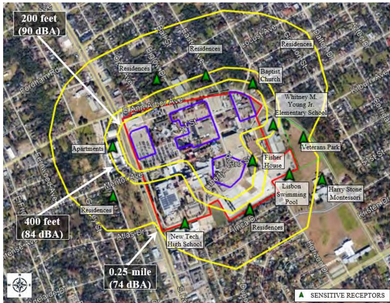
**Figure 3-4 Estimated Peak Construction Noise Level Contour Map**
