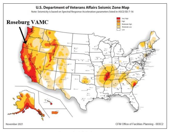
Figure 1-4 VA Seismic Zone Map
