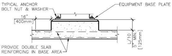
SECTION A-A (BASE POURED WITH FLOOR SLAB)
