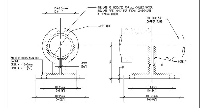
NOTE: WHERE USED FOR COPPER TUBE OR PIPE, BRAZE TO FABRICATED STEEL ANCHOR
