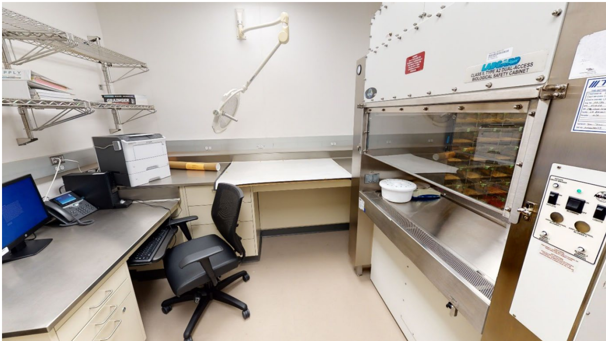
Image A.10 Small animals received at the Rocky Mountain VAMC R&D Facility are examined in this room and then moved through the biological safety cabinet pass-through into quarantine. (Note: Disparities between the plan and execution of this room resulted in it not being used as much as would be preferred.)
