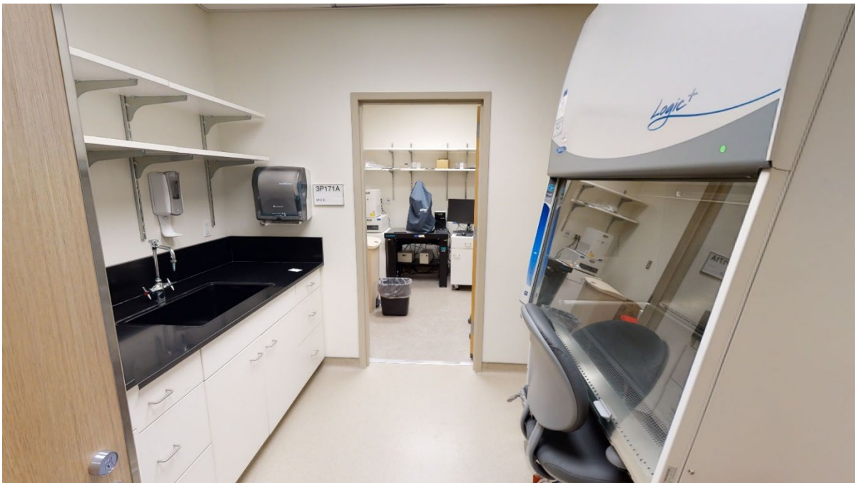
Image A.15 The two-room configuration of the Tissue Culture Room at the New Orleans VAMC R&D Facility facilitates maintenance of negative air pressure.
