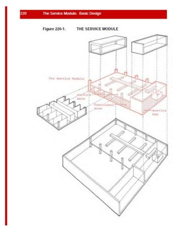
**Service Zone:** The horizontal layer or building volume between the bottom of a finished ceiling and the top of the finished floor immediately above; and the adjoining service bay. See Interstitial Space.
